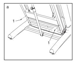
Lower the treadmill (see HOW TO LOWER THE TREADMILL FOR USE on page 20). Remove the four indicated #8 x 3/4" Screws (1), and remove the Motor Hood (75).
